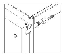
Hermetically close the door again by tightening the bolts (2) until the door compresses the braided seal.
