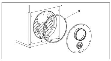
On completion of cleaning, follow the above steps in the reverse order to refit all removed parts.
