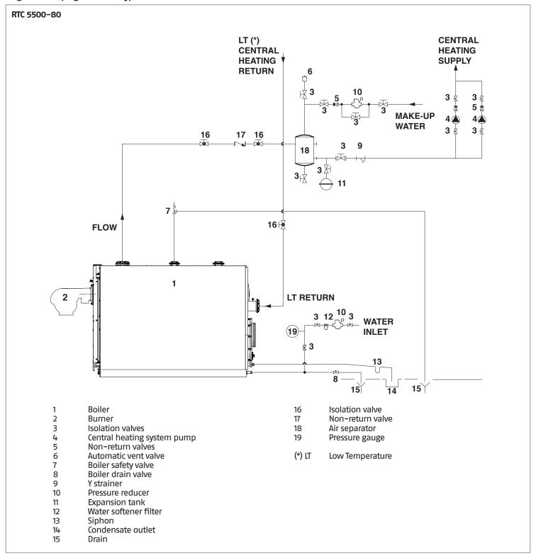
Single Boiler Combination Heating & Domestic Water Plant
