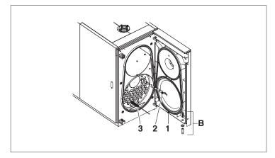
$oldsymbol{\Lambda}$  The first time opening the door, remove the spare hinge assembly (B) (bushing, bolt, and washer) opposite the pivot side of the door.
