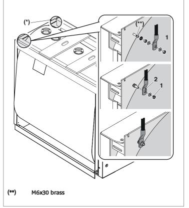
Another hole (\*) in the left side of the boiler head can also be used to ground the appliance. If you wish to use this hole for the earth connection, remove the terminal fittings from the right of the head and move them to the left grounding point.
