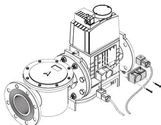
The seal control function is included on Burner Digital Management System, it is only necessary to add the PVP kit on the gas train.
