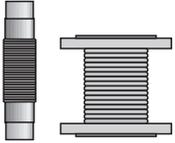
Anti-vibrating joints to damp vibrations and facilitate application of the gas train to the gas distribution line are available in different sizes listed in the table below.
