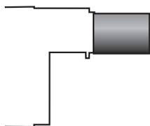
"Standard head" burners can be transformed into "extended head" versions, by using the special kit.
