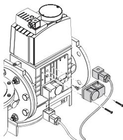
The seal control function is included on Burner Digital Management System, it is only necessary to add the PVP kit on the gas train. The PVP is included as standard equipment on RS 810-1000-1200-1300-1600-2000/E-EV FGR models.
