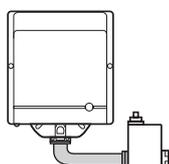
There is a special kit available that can be used to install the burner turned 180°. This kit is designed to ensure the gas train valve properly.
