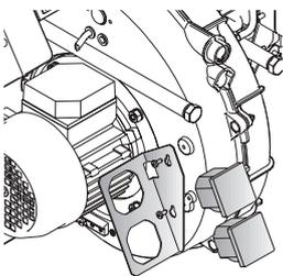
To measure the burner working time a hours counter kit is available.
