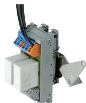
A volt free contact kit is available for installation onto the burner. It can be used for a remote interface between burner operating signals. Every burner can be equipped with a single kit to remote the flame presence signal and the burner lockout indication.
