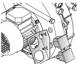
To measure the burner working time a hours counter kit is available.
