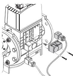
The seal control function is included on Burner Digital Management System, it is only necessary to add the PVP kit on the gas train. The PVP is included as standard equipment on RS 130/E-250/E-EV MZ and RS 190/E models.
