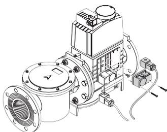
The seal control function is included on Burner Digital Management System, it is only necessary to add the PVP kit on the gas train. The PVP is included as standard equipment on RS 1300-1600-2000 models.
