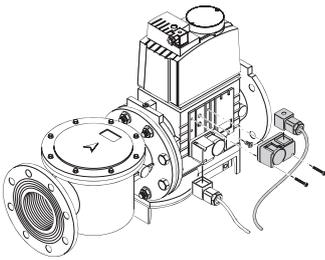
The seal control function is included on Burner Digital Management System, it is only necessary to add the PVP kit on the gas train. The PVP is included as standard equipment on RS RS1300-1600-2000 models.
