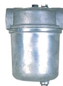
To solve problems of air or water in the oil circuit a special filter/degassing unit is available, made up of aluminium cover, plastic tank, stainless steel filtering cartridge, air release cap and water purge valve. It is available singularly.
