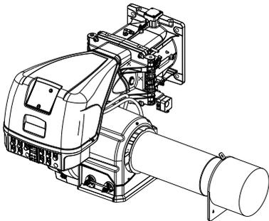
When burner is used in dusty environment, in order to prevent the possible ingress of foreign elements in the air circuit, a filter is available as accessory to be installed in the air intake side of the burner.
