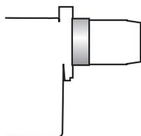
Using the special accessories, the burner can be pulled back to reduce head penetration into the combustion chamber.
