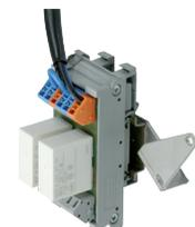
A volt free contact kit is available for installation onto the burner. It can be used for a remote interface between burner operating signals. Every burner can be equipped with a single kit to remote the flame presence signal and the burner lockout indication.
