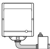
There is a special kit available that can be used to install the burner turned 180°. This kit is designed to ensure the gas train valve properly.
