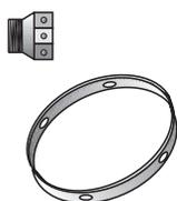
For burning LPG gas, a special kit is available to be fitted to the combustion head on the burner as shown in the following table.
