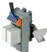
A volt free contact kit is available for installation onto the burner. It can be used for a remote interface between burner operating signals. Every burner can be equipped with a single kit for a remote check of the flame presence signal and the burner lock-out indication.
