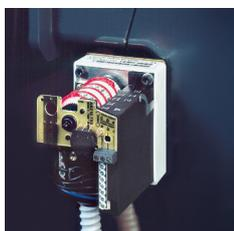
Depending on the servomotor fitted to the burner, a three-pole potentiometer (1000 Ω) can be installed to check the position of the servomotor.
