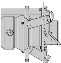
For burning LPG gas, a special kit is available to be fitted to the combustion head on the burner, as given in the following table.
