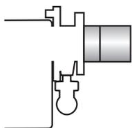
Burners "standard head" can be transformed into "extended head" versions by using the special kit. Here the KITS available for the various burners are listed, showing the original and the extended lengths.
