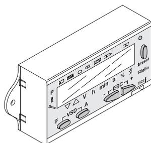
The AZL 21 LCD display Kit is suitable to be connected to the LME 71 control box in order to get indication of the operating status, to activate the diagnostic functions and to change the password-protected parameters (carried out only by qualified personnel)
