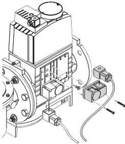
The seal control function is included on Burner Digital Management System, it is only necessary to add the PVP kit on the gas train.
