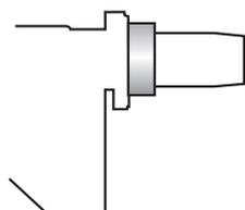
By using the special accessories, the burner can be with-drawn to reduce head penetration into the combustion chamber.
