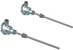
The kit includes two temperature sensors: one for air and one for exhaust gas detection. They must be wired to oxygen control kit interface to allow the LMV 52 efficiency calculation. The value is showed on AZL display.
