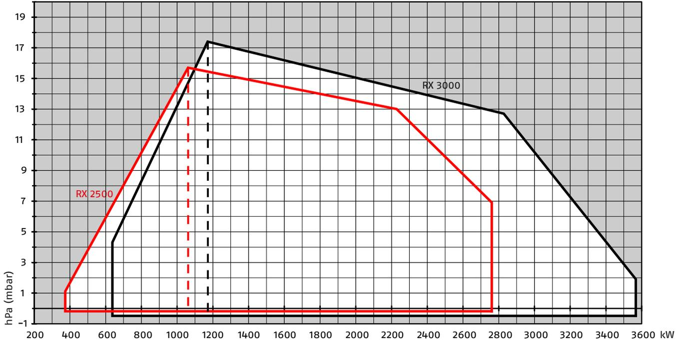
Please note: it is important to be aware that in order to achieve an ULTRA low NOx emission performance, it is required to work with a high excess air; as consequence the combustion chamber back pressure could increase up to roughly 30% more.
