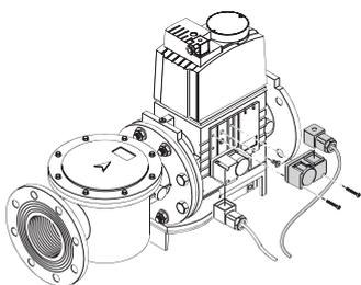
The seal control function is included on Burner Digital Management System, it is only necessary to add the PVP kit on the gas train. The PVP is included as standard equipment on RLS 1300-1600-2000 models.
