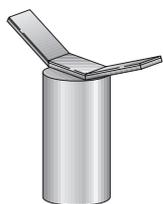
For easier maintenance, a mobile burner support has been designed, which means the burner can be dismantled without the need of forklift trucks.
