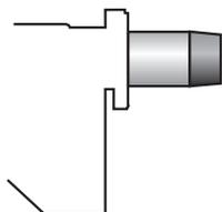
Burners standard head can be transformed into "extended head" versions by using the special kit.
