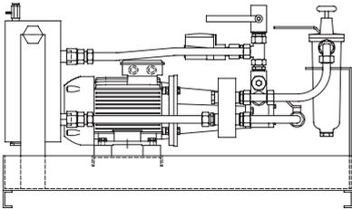
The RLS 1600 and RLS 2000 burners must be combined with a pumping unit suitable for the output to be produced. The pump unit models available in combination with these burners are indicated in the table below.
