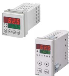
To obtain modulating operation, the RS/M BLU series of burners requires a regulator with three point outlet controls. On RS 25/M - 35/M BLU the regulator is connected to the burner electrical wiring by plug-in system in order to make the connection easier and faster.
