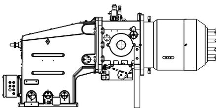
DN 80 gas connection from below (for gas versions). Elbow adapter DN 80 required.
