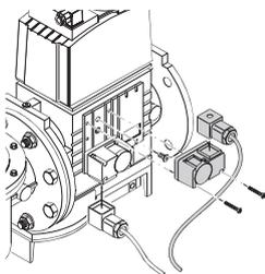
The seal control function is included on Burner Digital Management System, it is only necessary to add the PVP kit on the gas train. The PVP is included as standard equipment on RS 810/E-EV BLU models.
