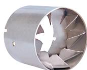
The end cone turbulator disk reduces the flame length. It is suitable for oven application (CO emissions) and short boiler chamber.
