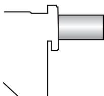
This kit can be used to prevent combustion instability which could arise with particular heat generators. To extend the adaptability of Gulliver BSDF burners to any sort of application, alternative combustion heads have been developed. These heads cause a very limited increase in NOx emissions, due to the slower air flow.
