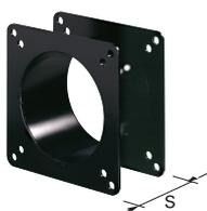
If burner head penetration into the combustion chamber needs reducing, varying thickness spacers are available, as given in the following table:
