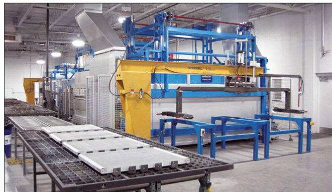
Controlled Atmosphere Brazing Furnace
