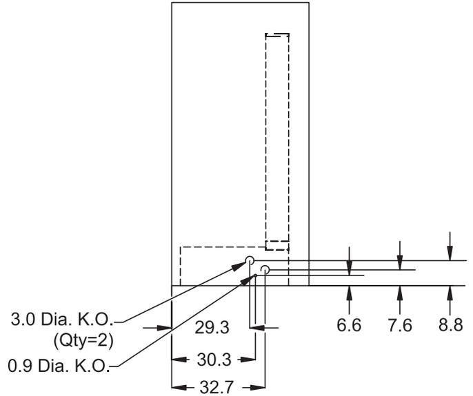
**Figure 31: Main Control Panel/Discharge Plenum, RFS/RPS 045C to 075C or RAH 047C**
