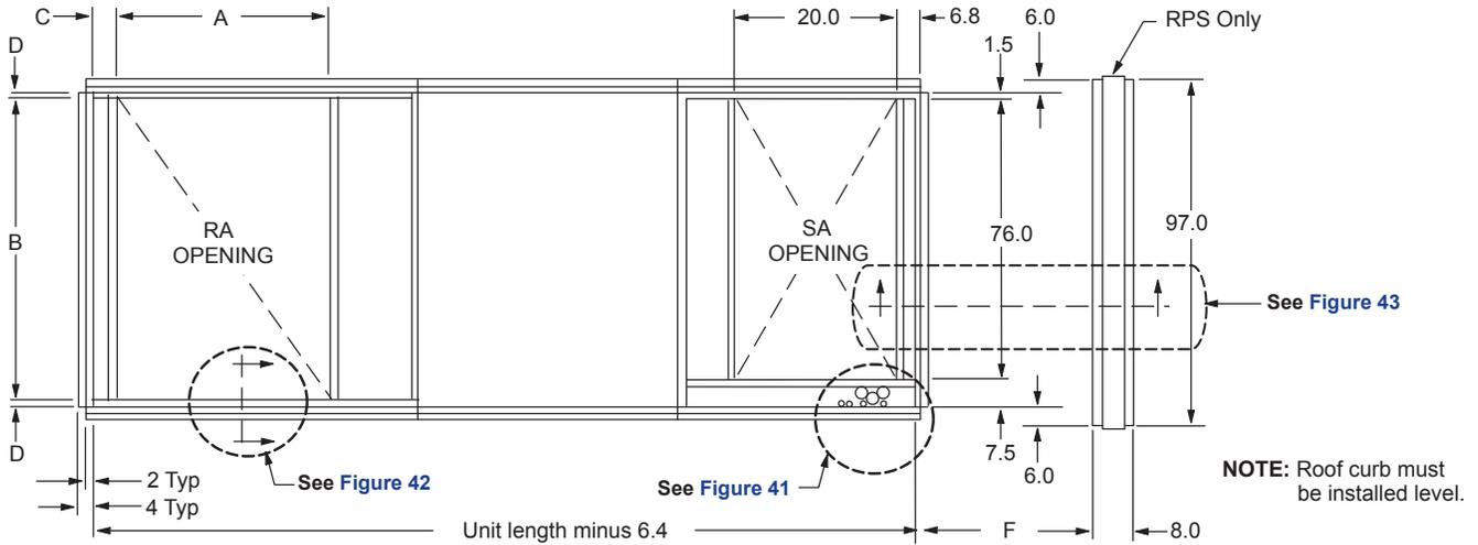
Figure 38: RFS/RPS 015C to 040C Roof Curb, (with blank compartment)
