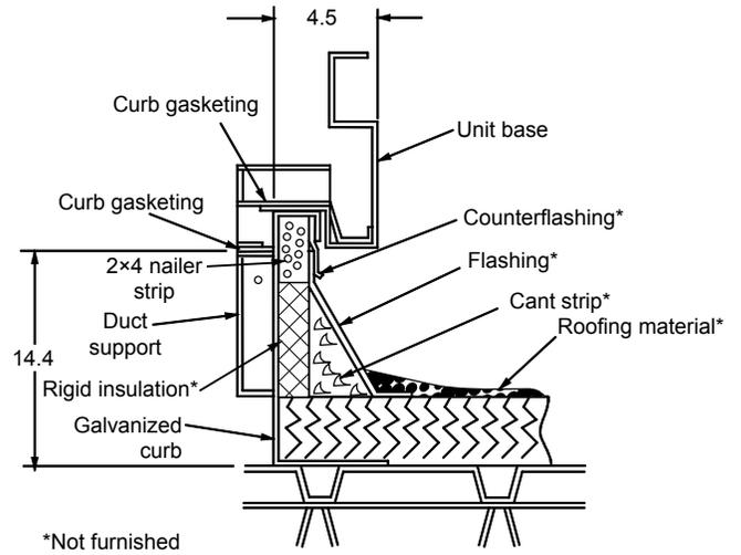
Figure 43: RFS/RPS Curb Section B-B
