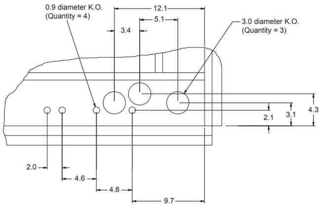
Figure 42: RAH/RDS/RFS/RPS Curb Section A-A
