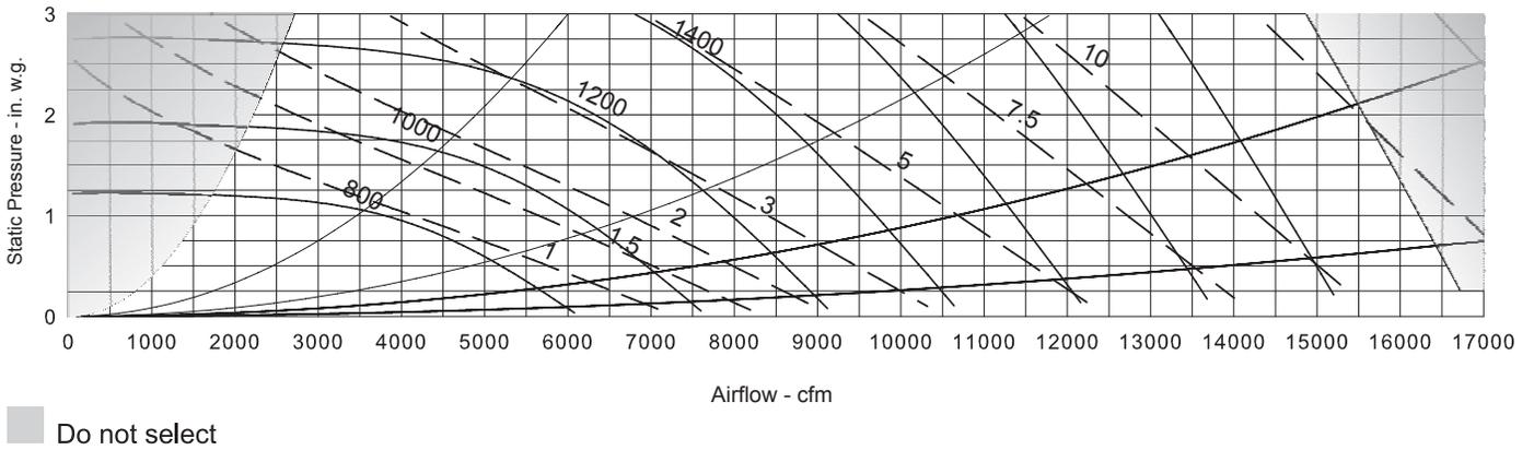
Figure 24: RDT/RFS/RPS 045C to 075C or RAH 047C; 40 in. Airfoil Return Fan
