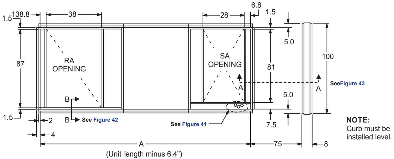
Figure 40: Roof curb, RPS/RFS 045C to 075C (with blank compartment)
