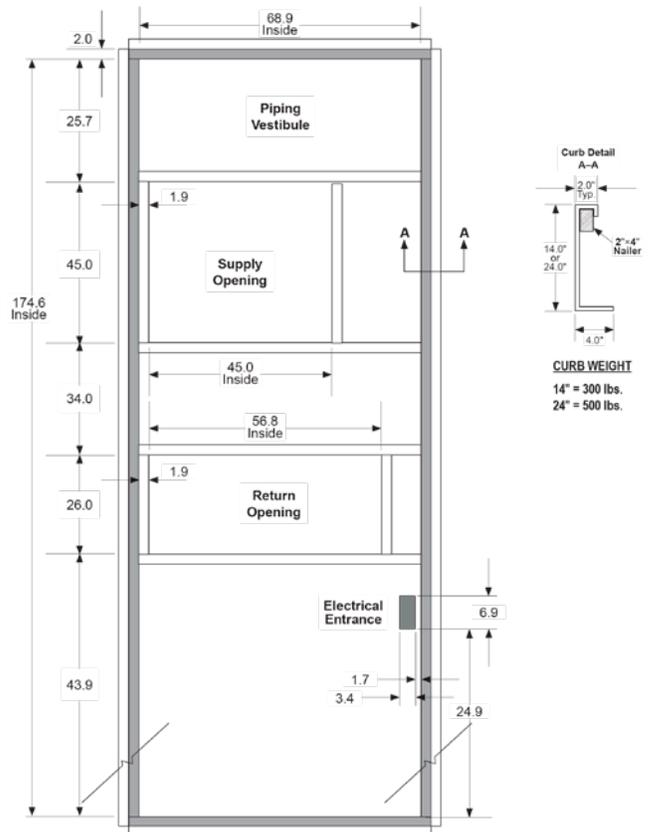
Figure 13: Roof Curb Assembly (DAH A07, A11, A15—A21) with CORE ERV
