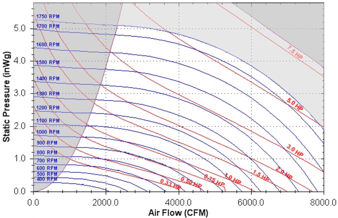
Figure 20: Fan Curve – DDPL-16 – Size 15–21
