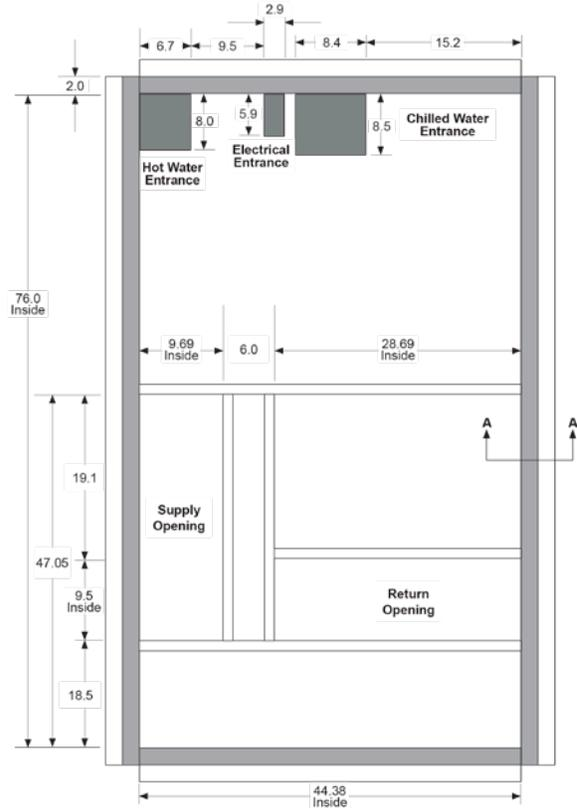
Figure 11: Roof Curb Assembly (DAH A07-A11)<sup>1</sup>
