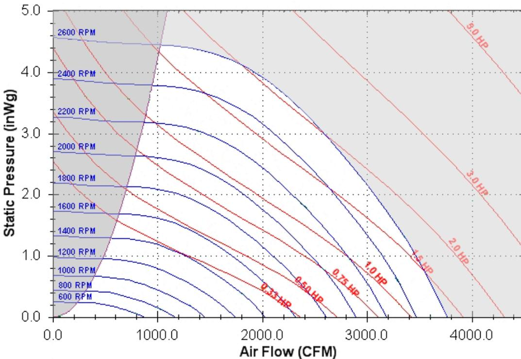
Figure 18: Fan Curve – 16 inch Fan
