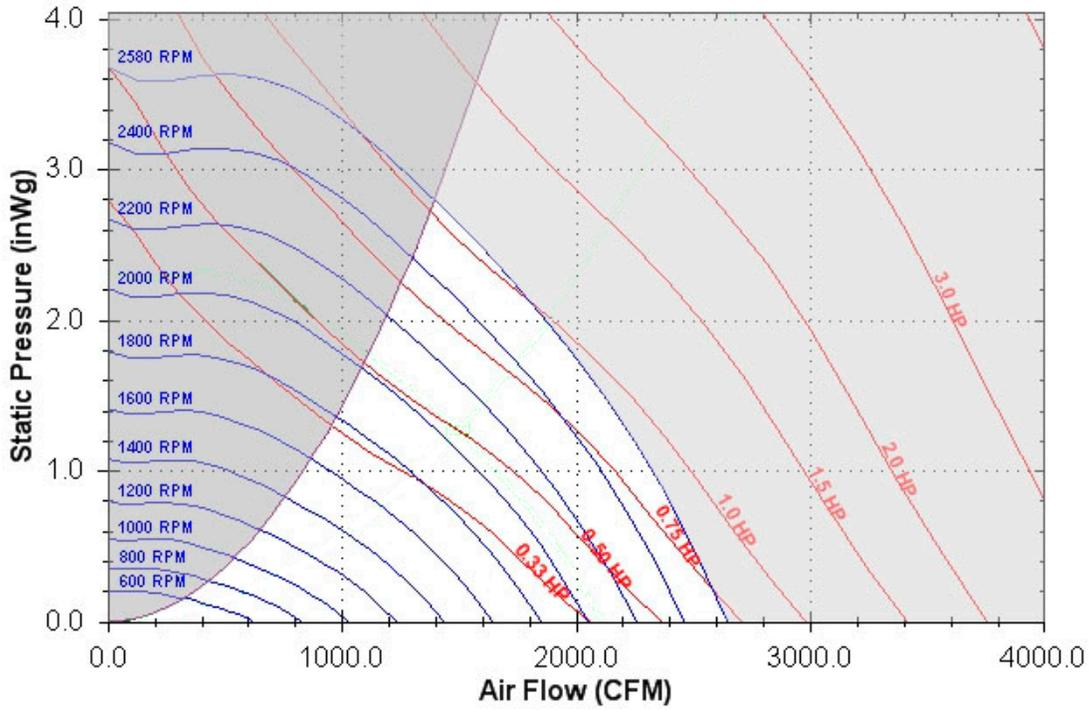
Figure 17: Fan Curve – 14 inch Fan
