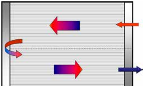
Figure 2: Typical 2-Pass Construction
