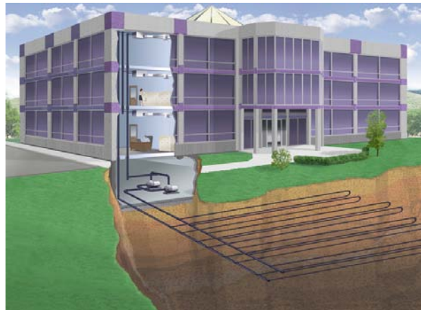
Figure 10: Horizontal loop application
