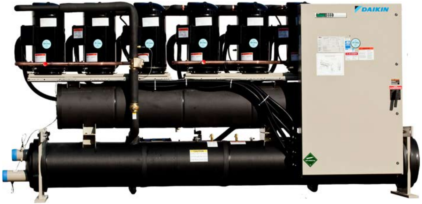
On the cover: Templifier Model TGZ120 with standard four-pass condenser. Shown less piping insulation for clarity. Above: Model TGZ190 with standard 4-pass condenser with optional left-hand condenser connections.
