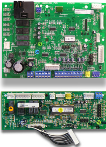
Figure 3: MicroTech III SmartSource unit controller and I/O expansion module
