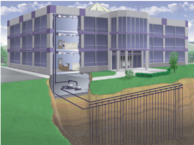
Figure 18: Vertical loop application
