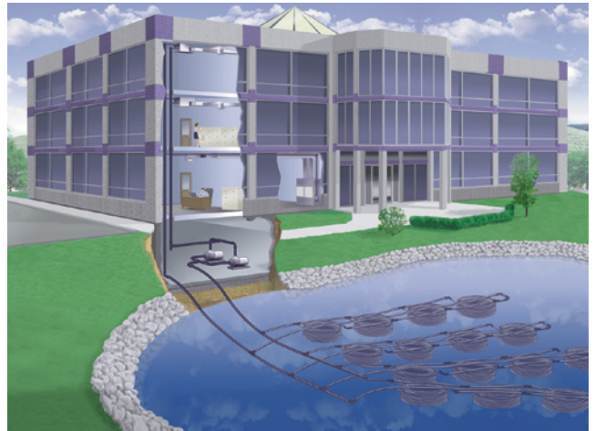
Figure 20: Surface water loop application
