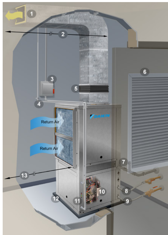
Figure 21: Typical VFC installation – closet, non-ducted return
