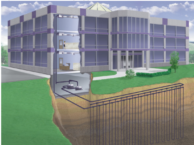
Figure 17: Vertical loop application
