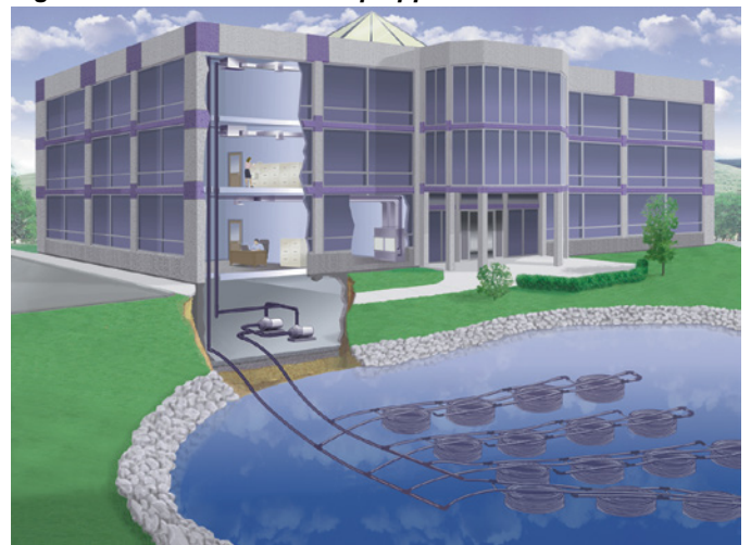
Figure 19: Surface water loop application
